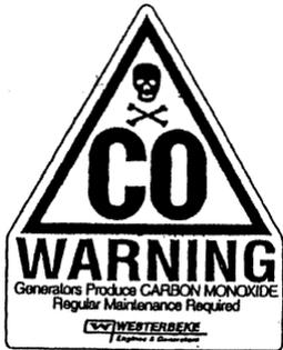
A WARNING DECAL is provided by Westerbeke and should be fixed to a bulkhead near your engine or generator. Westerbeke also recommends installing CARBON MONOXIDE DETECTORS in the living/sleeping quarters of your vessel. They are cost affective and easily obtainable at your local marine store.
