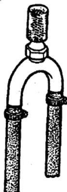
**NOTE:** A siphon-break requires periodic inspection and cleaning to ensure proper operation. Failure to properly maintain a siphon-break can result in catastrophic engine damage. Consult the siphon-break manufacturer for proper maintenance.
