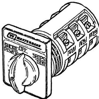
Set the transfer switch shown in the diagram to the **OFF** position. This switch prevents simultaneous connection of shore power to generator output.
